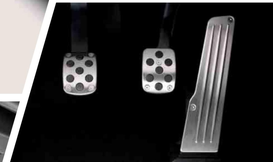
**ALUMINIUM PEDALS WITH AN ANTI-SLIP RUBBER AREA AND FOOTREST.**
